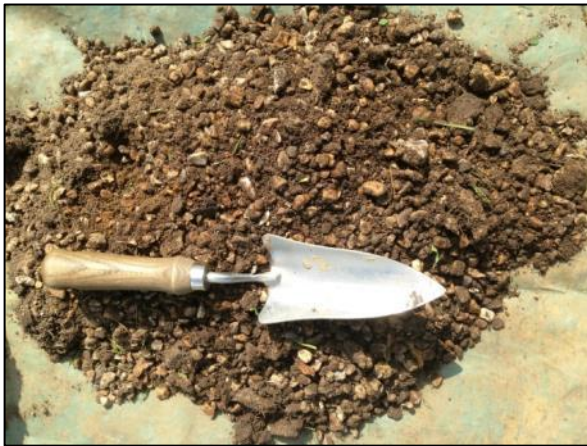
Figure 11. Gravel contaminated with soil.
