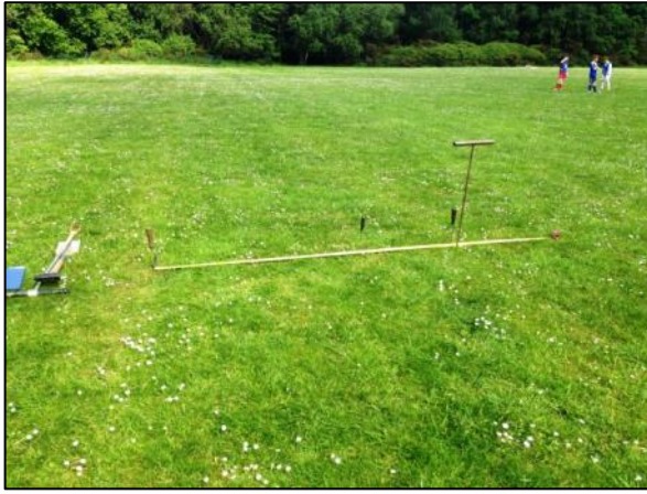
Figure 9. Locating drains using a spiked probe.
