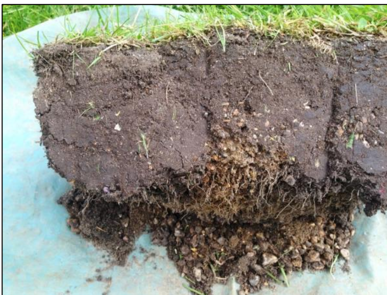
Figure 13. 170 mm of topsoil – TP1.
