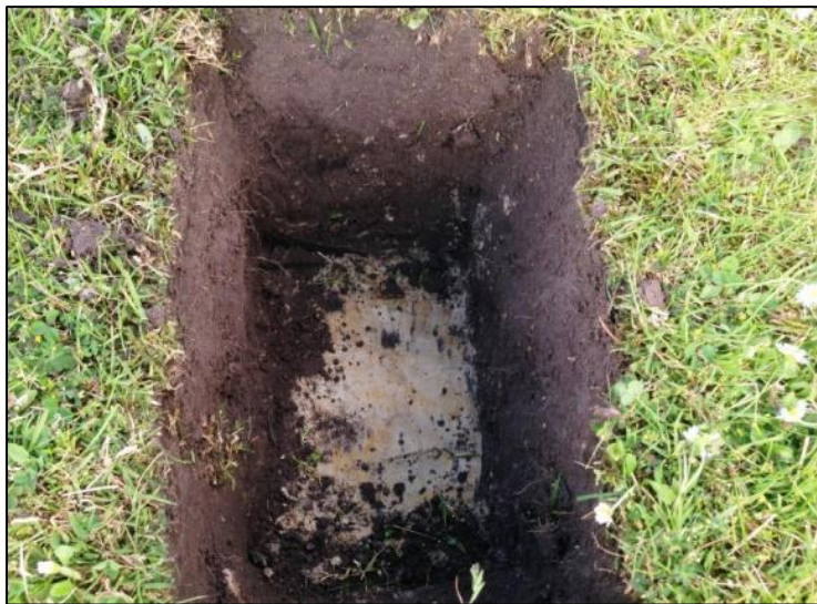
Figure 15. 200 mm of topsoil over sand – TP2.
