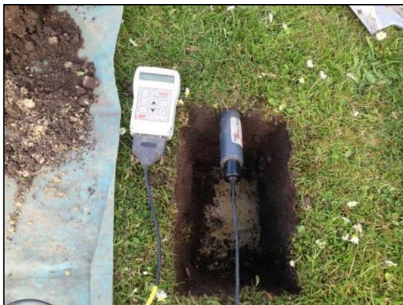
Figure 17. Measurement of water content using a Theta Probe.
