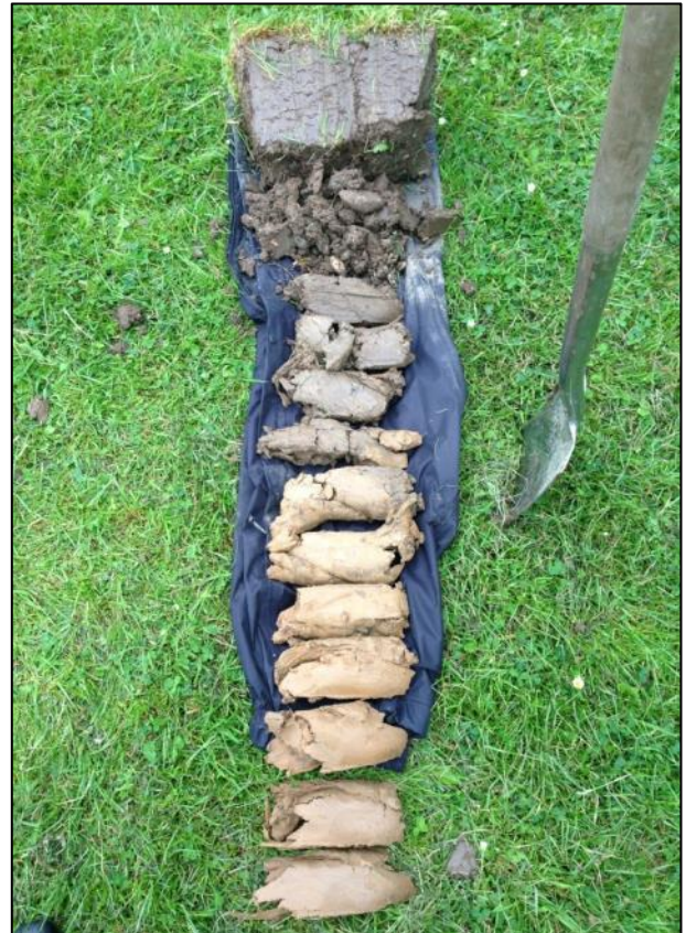
Figure 9 TP1 400 mm CLAY LOAM topsoil over plastic CLAY subsoil, mottled in appearance to a depth of 1000 mm indicative of saturated conditions.
