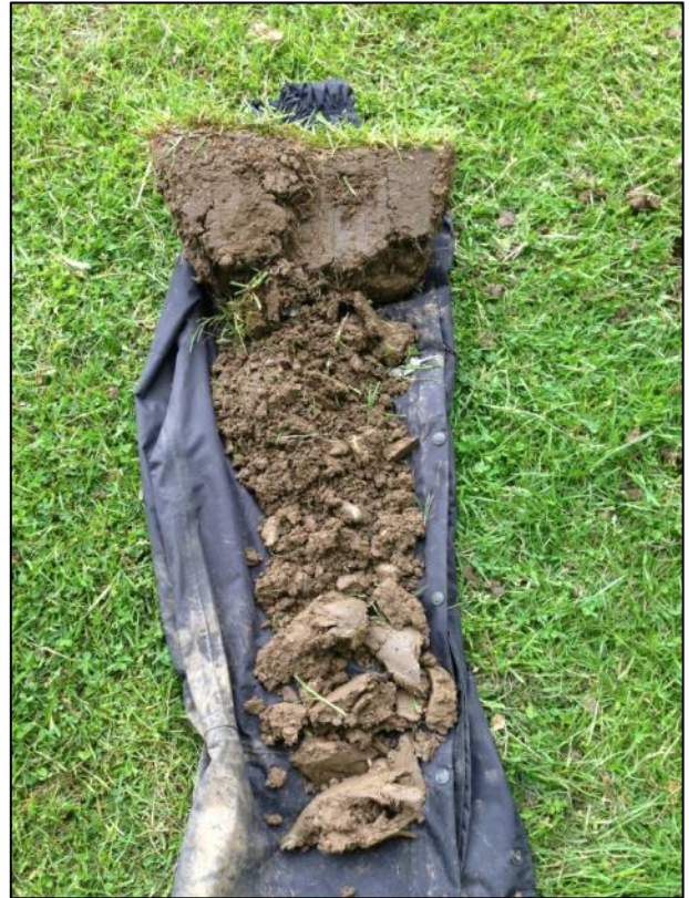
Figure 11 TP2 comprised 450 mm of CLAY LOAM topsoil (very stony).
