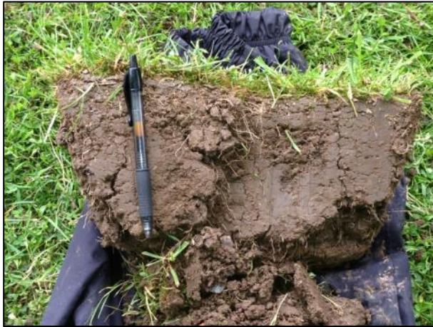
Figure 10 TP2 Poorly structured CLAY LOAM topsoil
