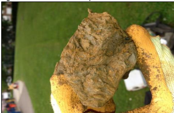
Figure 8 Example of mottled sub soil (TP1)
