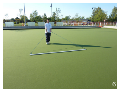
Testing of surface regularity by the WB test house
