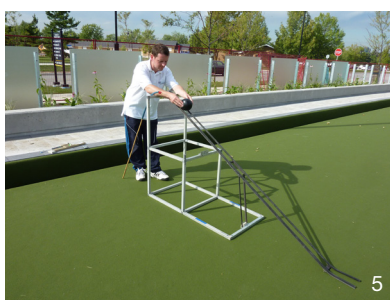
Testing of green speed by the WB test house
